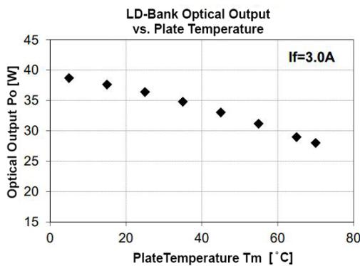
Figure 10. The efficiency of the output power related to the temperature of the module.
