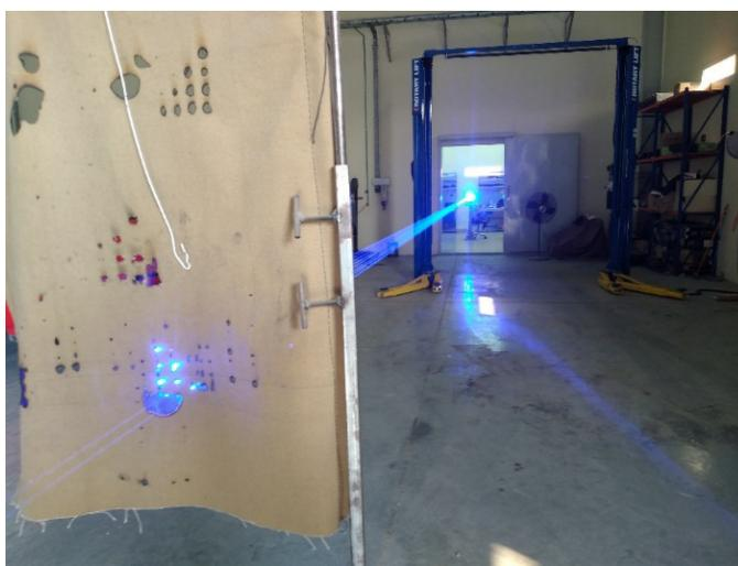
**Figure 20.** The Canvas fabric burned by the laser beam from a distance of 55 metres in a few minutes.
