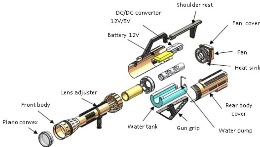
Figure 14. The different parts of the cannon prototype.
