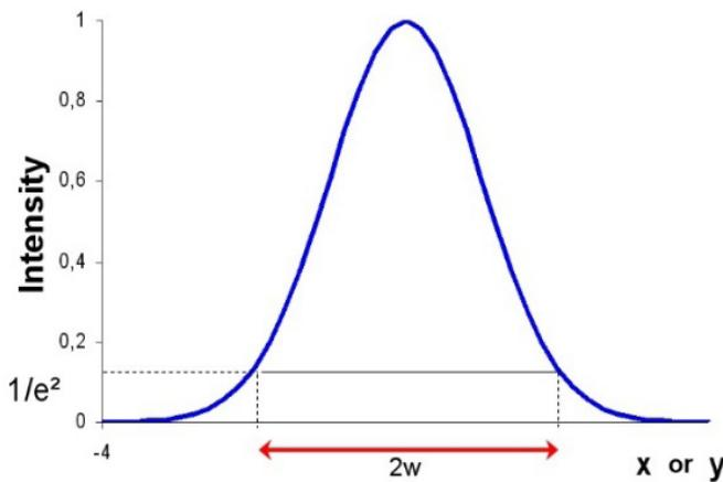
Figure 4. Intensity profile of Gaussian beam.
