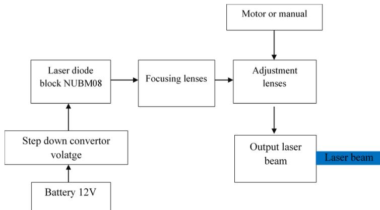
Figure 7. Block diagram of laser cannon.
