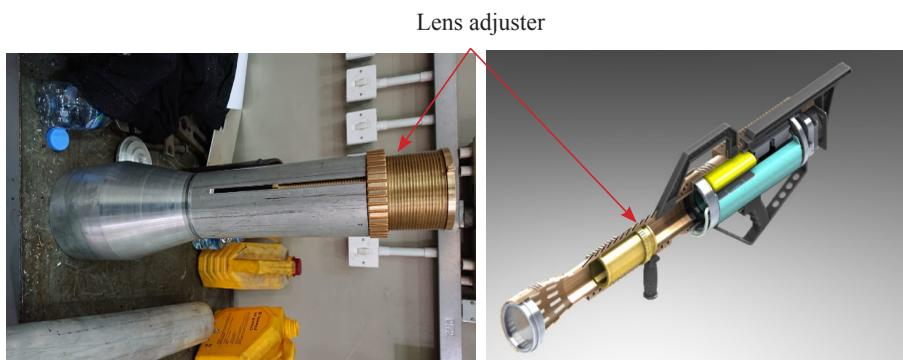
Figure 16. The mechanism to adjust the laser beam.
