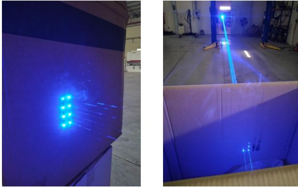
**Figure 21. The laser beam burns holes in the hard carton in 20 seconds.**
