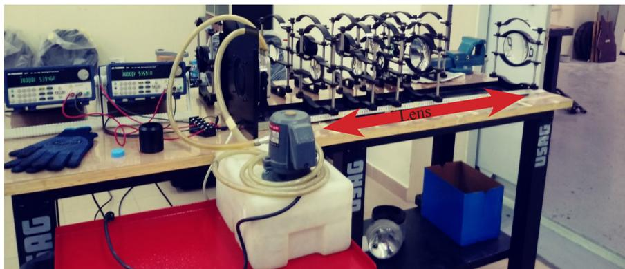
Figure 13. Gaussian Beam propagation through multi lenses.
