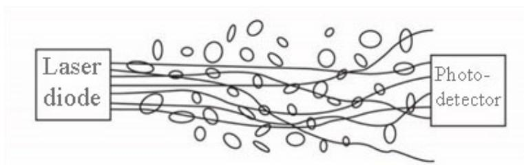
Figure 6. Turbulent cells through the whole optical path.
