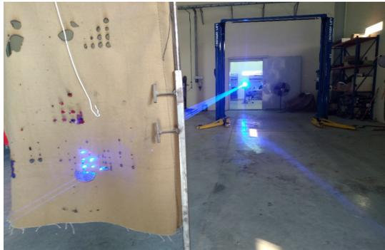
Figure 18. The experiment shows it burns holes through clothes in a few seconds.
