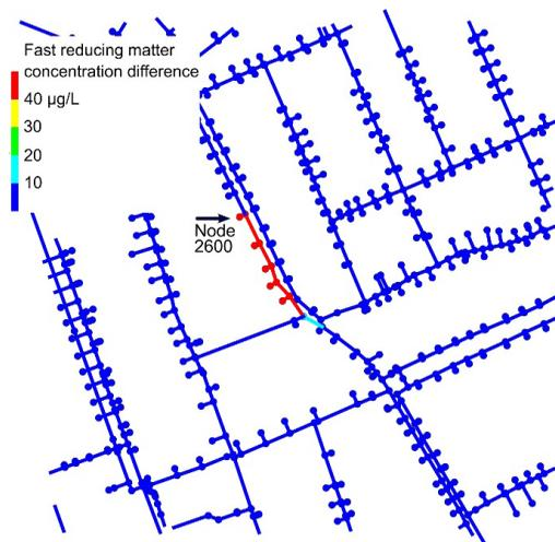
Figure 6. Difference in fast reducing matter concentrations when contamination is present compared to normal operation.
